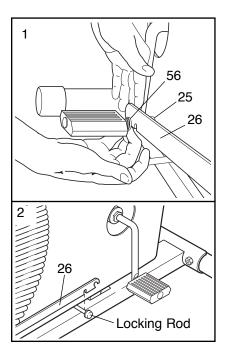
Clip the Link Arms (26) onto the lock rod as shown in drawing 2.
